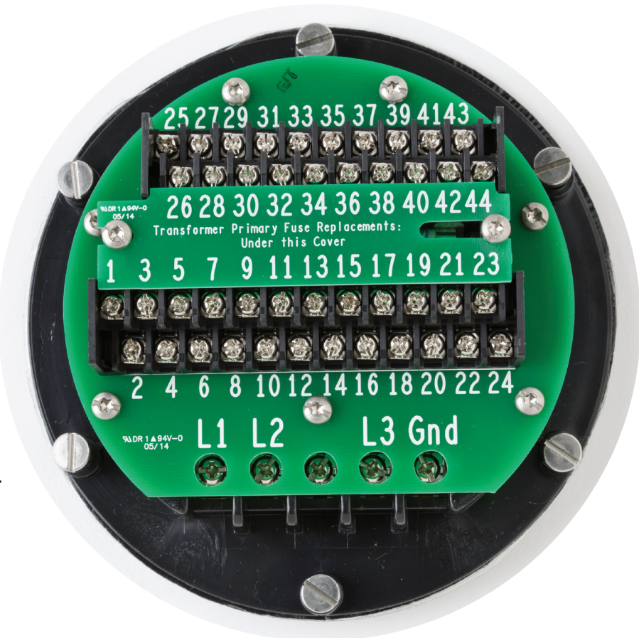
Figure 6: Separate Terminal Chamber (STC) with Spade Lug Data
