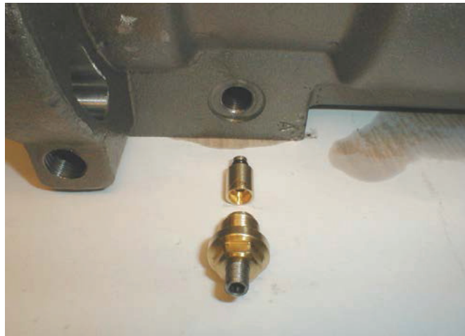
Figure 15 Crossover Valve and Seat Removed
