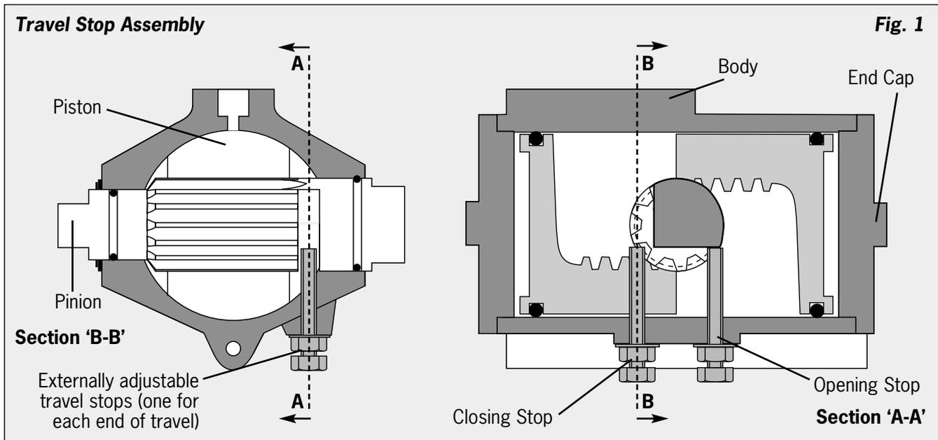
the hole. Having removed the coil from one end cap, repeat the operation with the other end cap. When both coils have been removed, push out the end caps part way by rotating the pinion. Remove the end caps by pulling them free from the body, avoiding any 'cocking' of the end caps.
