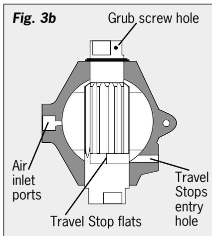
approximately 30°. If Travel Stops are fitted, the grub screw hole on the top of the pinion must be facing away from the air inlet ports (as shown in Fig. 3b). This ensures that the machined Travel Stop Flats on the base of the pinion are in the correct position.
