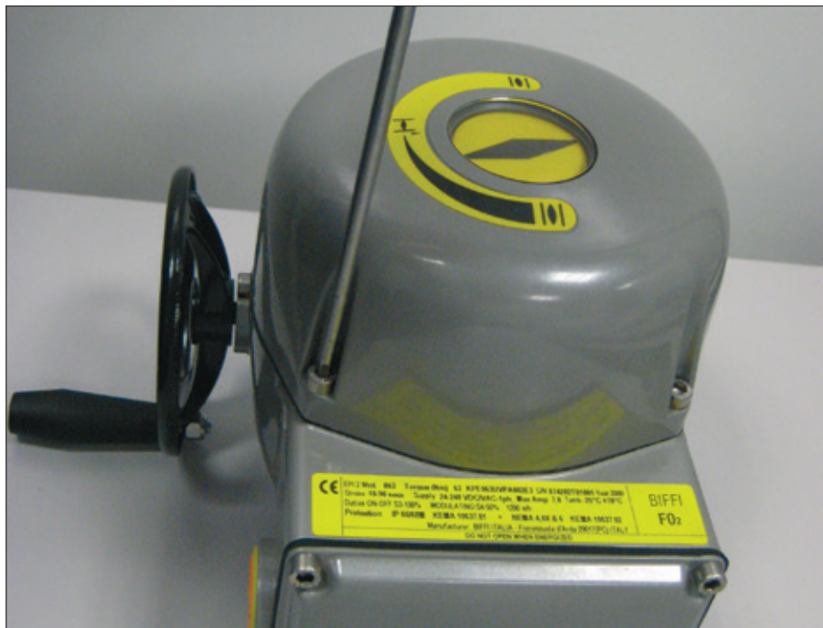
FIGURE 14 - Removal of the control unit cover.
