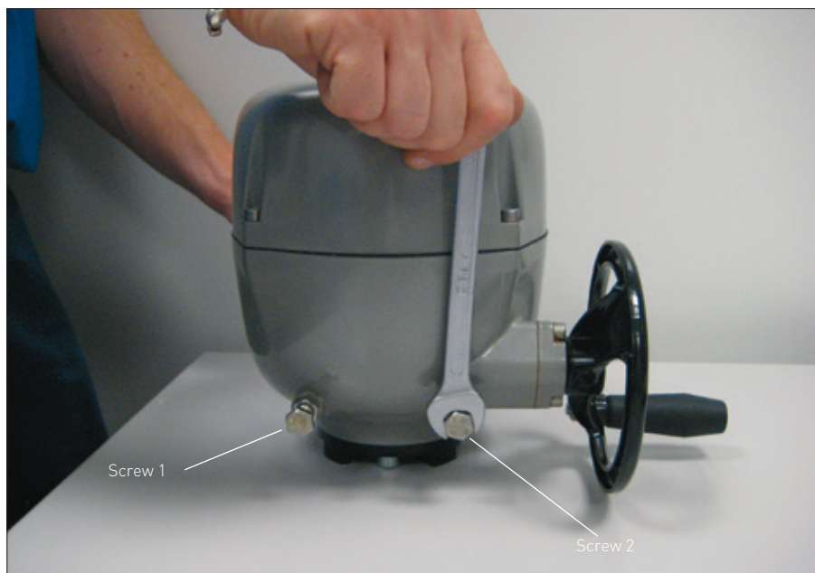
FIGURE 7 - Setting of the mechanical stop.
