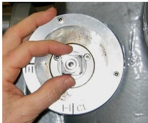
5) Rotate the indicator nut clockwise until it blocks at the end of threads; rotate a few degree counter clockwise until the flat surface is perfectly aligned with the CLOSE indication of the label.
