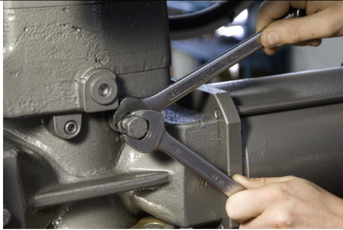
Setting the stop screw positioned on the actuator's carter
