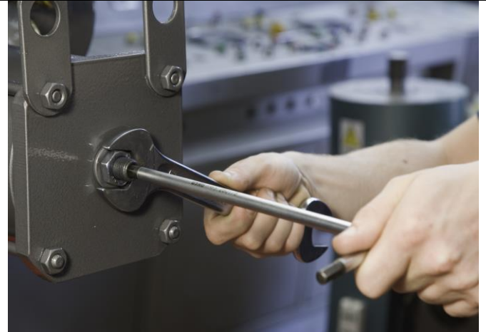
Setting the stop screw positioned on the spring cartridge end flange
