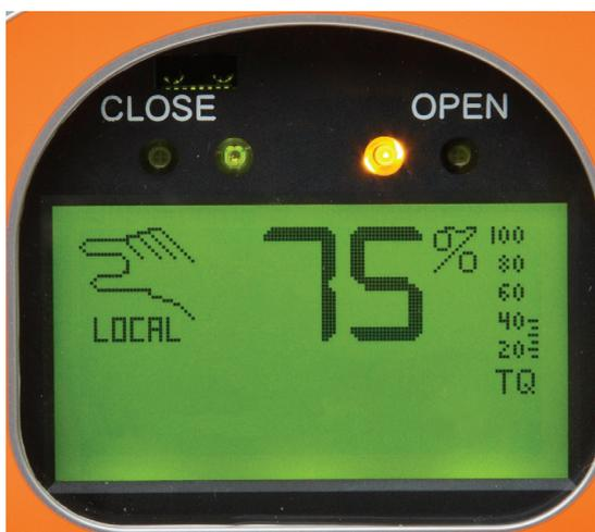
The valve has stopped and is 75% opened. The yellow LED is ON and the message center is clear.
