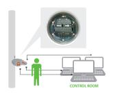
Separate Terminal Chamber. Dual sealed separate terminal chamber with highly legible terminal markings and pre-installed screws eases field wiring. Primary fuses accessible without opening controls compartments
