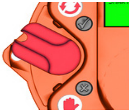
Figure 20 Selector Switch in Neutral Position (2)
