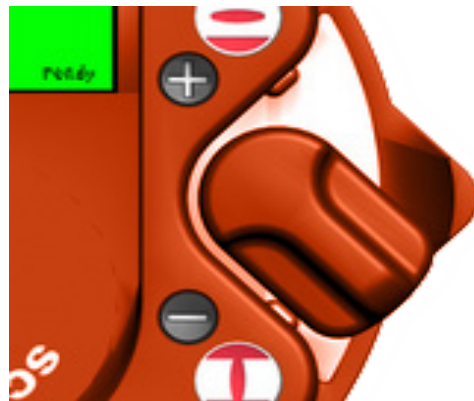
Figure 40 Full Switch Trip (it will jump to the end of the menu)
