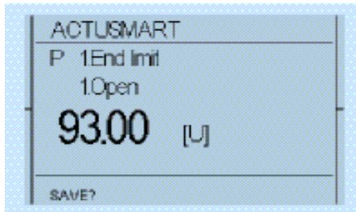
In order to confirm the end position (save), slightly flip up the selector switch and let it snap back to its neutral position.
