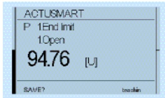
Manually move the actuator with the handwheel (see [Section 13.1](#) or [Section 13.6](#)) or by motor via the operating switch (black button) to the end position OPEN of the valve.
