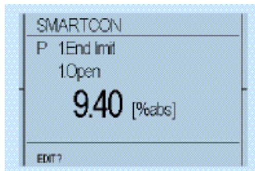
During operation, the displays shows the position of the actuator as a percentage, operation mode and status. When using the option identification, a customer-specific label is shown at the bottom of the display (e.g., PPS Number).
