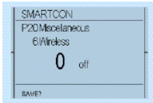
Use the control switch towards the characters to change the parameter ⊕ or ⊖ (see Figure 42 to Figure 45). After reaching the desired parameter value, confirm the value with the selector switch again, flip it slightly towards ✓, (see Figure 33 to Figure 35).
