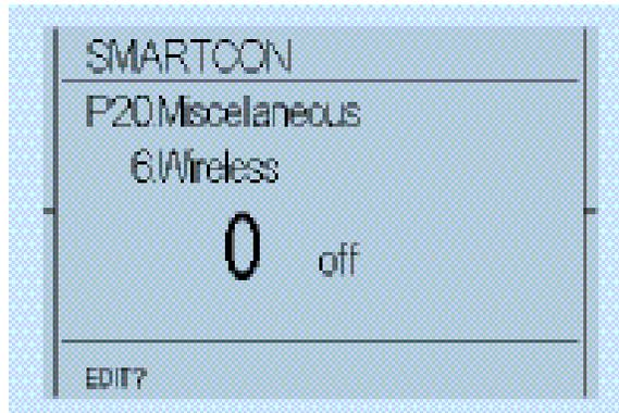
Confirm the selector switch with a slight flip towards ✓, (see Figure 33 to Figure 35) to change the selected parameter. To confirm this input readiness, the display changes from "EDIT?" to "SAVE?".
