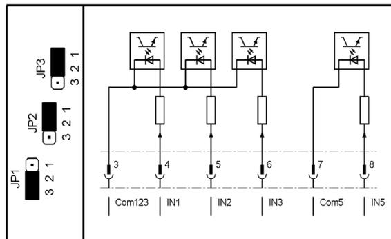
Jumpers JP1 to JP3 can be used to interconnect the binary inputs to groups with separate earths:
