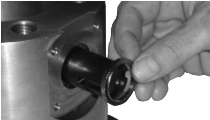
Figure 5. Insert Top End Ring
