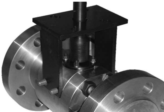
Figure 9. Position the Mounting Bracket
