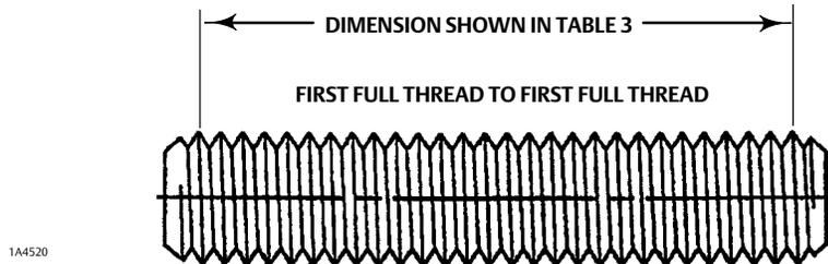
Table 3. Flange Stud Lengths Required for Flow Ring End of Fisher V150S Valves
