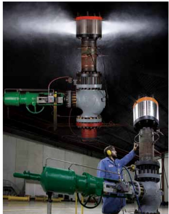
Noise testing of an NPS 12 vent diffuser.
