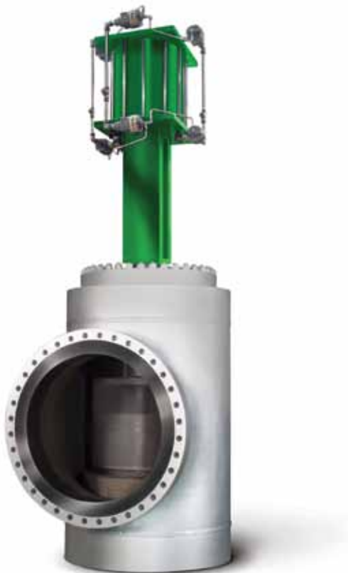
A Fisher noise-attenuation control valve can be built to meet the requirements of your application. The valve shown above is NPS 36 x 42 and contains a Fisher Whisper Trim III cage.
