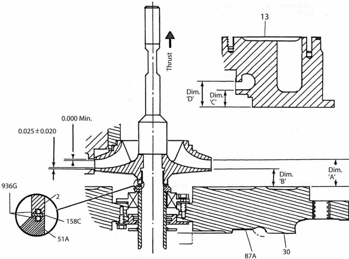
Figure 13. Shaft Loading Tool Installation
