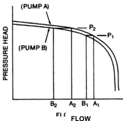
Figure 10. Parallel Units Common Valve
