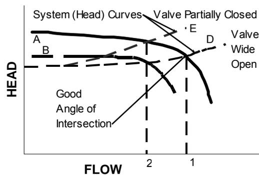
**Note:** The curve for pump A has a significant angle of intersection with system curves D and E. The system curve D could represent a system with the control valve wide open while curve E could represent the same system but with the throttle valve closed to reduce flow from flow 1 to flow 2. Pump curve B, on the other hand, will provide only flow 2, even with the control valve wide open
