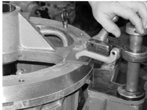
**Note:** "C" clamps can be utilized to perform this task. Be sure to protect the housing faces from any clamping damage.
