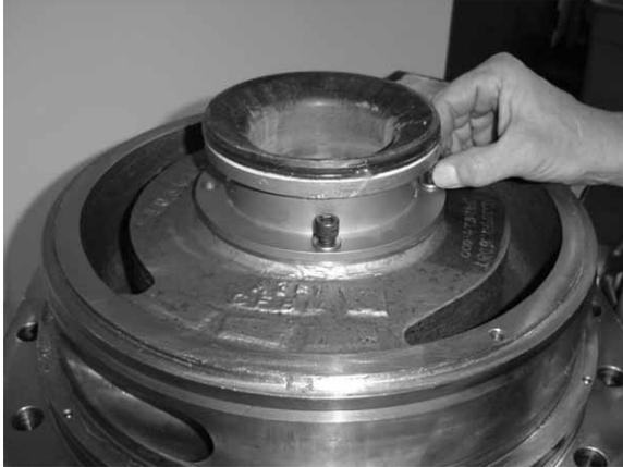
Removing the bolts from the inducer housing.
