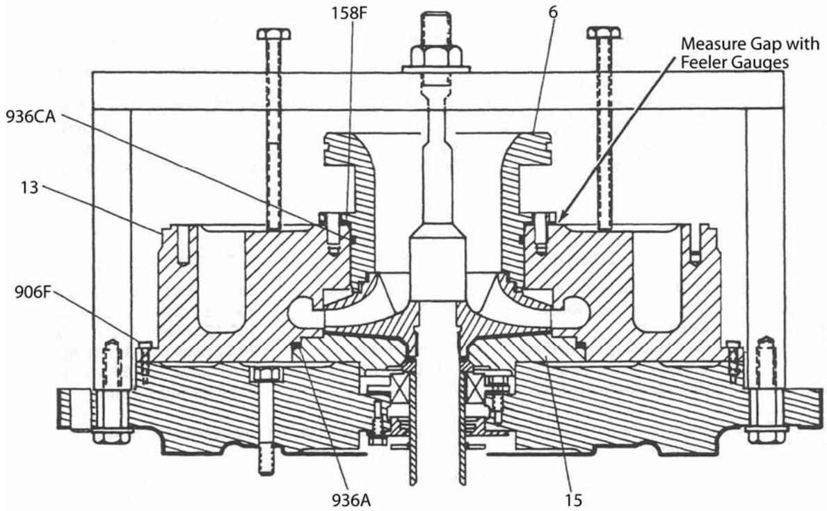
Figure 15. Inducer Housing Shim Adjustment
