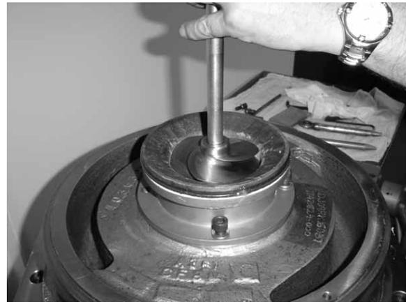
**Note:** When working on a pump with a tapered inducer, the inducer must be removed before the diffuser can be removed from the seal housing.
