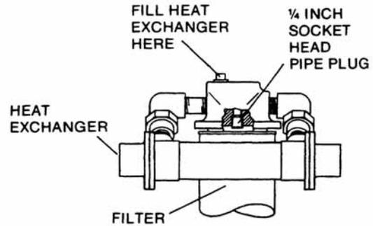
The MA01AA01 Model requires a 1/4" socket-head pipe plug in the filter manifold when using the gearbox heat exchanger. The plug must be removed when the heat exchanger is not being used.
