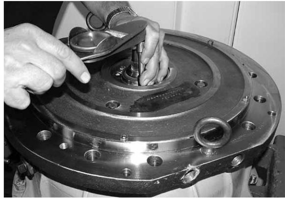
**Note:** Torque process seal hex head screws to 95-102 in-lbs.
