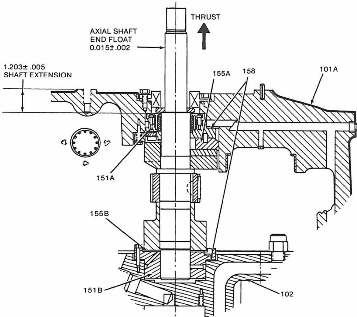
**Note:** Shims (158) are adjusted to obtain noted shaft end float and noted shaft extension. Shaft extension must be checked with thrust in noted direction. Measurements are made with dry (no oil) bearings.
