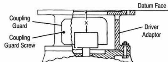
2. Determine the end gap (the distance between each coupling hub) for the size of coupling provided. Refer to the Coupling Specifications tables in the Specifications section of this manual for specific measurements.
