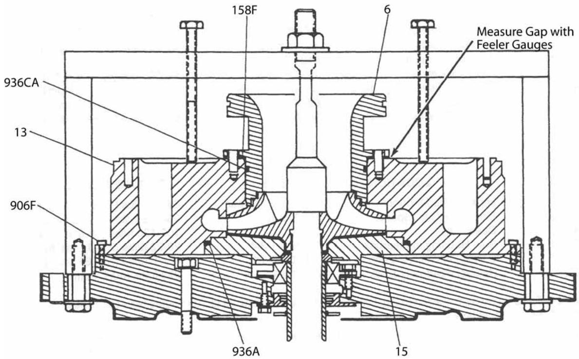
Figure 15. Inducer Housing Shim Adjustment
