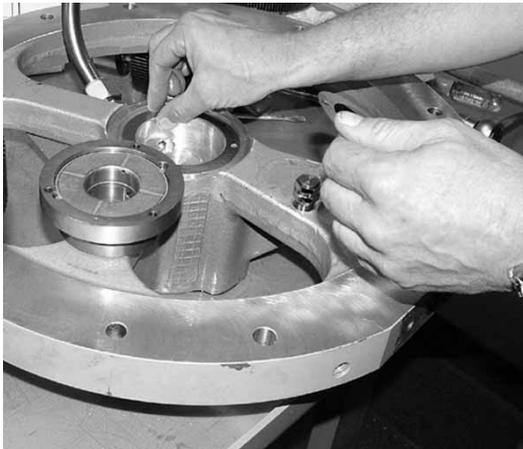
Re-install the upper journal bearing into the bearing plate.
