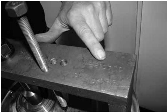
**Note:** *Torque values are shown on the tool. 25 ft-lb for standard tilt pad thrust and 50 ft-lb for high thrust glacier bearings.*
