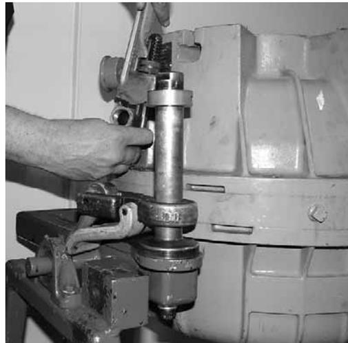
Use a pipe wrench to remove the fitting.
