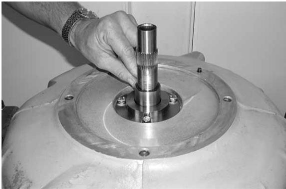
**Note:** If using Teflon or graphoil o-rings, do not install any of the o-rings until all measurements have been taken,
