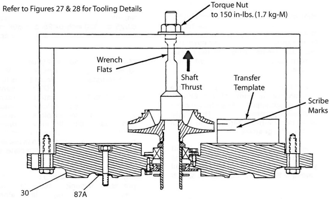
Figure 14. Inducer Housing Adjustment
