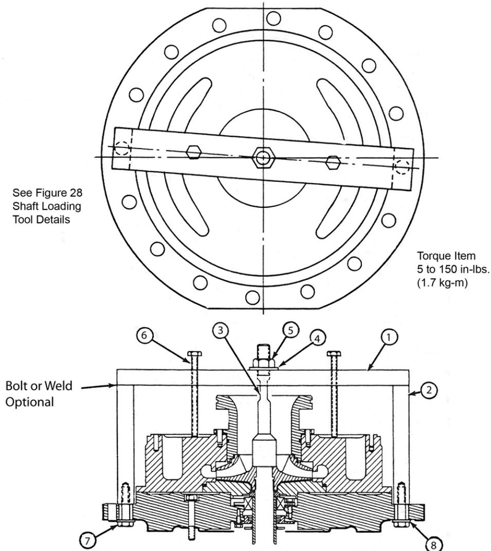
Figure 19. Shaft Loading Tool Details
