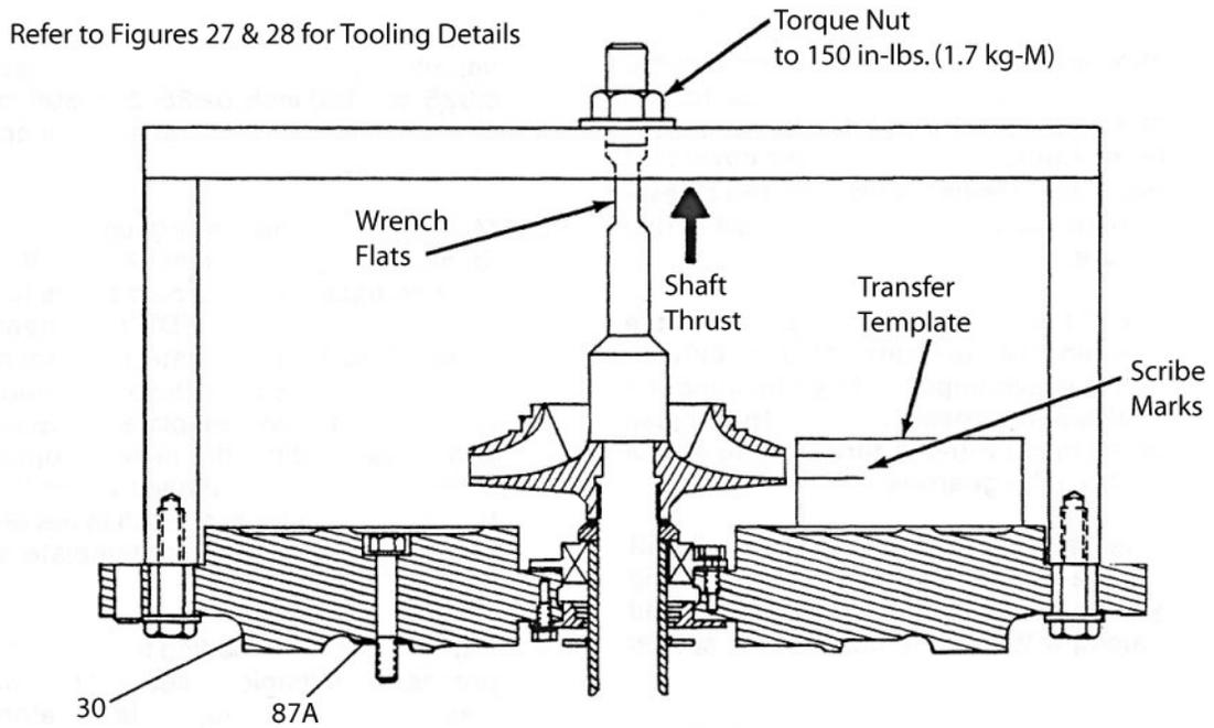
Figure 14. Inducer Housing Adjustment
