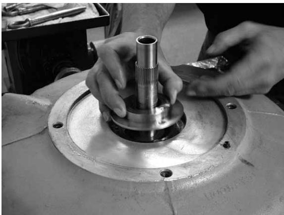
Use extraction tools to remove the rotating face.
