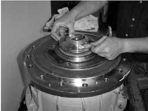
The impeller can be removed using two screwdrivers to pry up gently on opposite sides.
