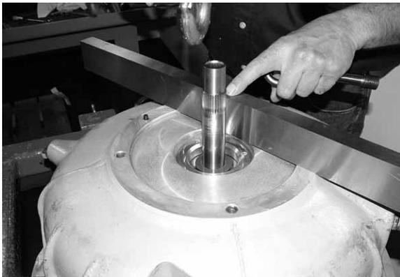
**Note:** Tolerances for shaft shoulder height are  $1.203 \pm 0.005$
