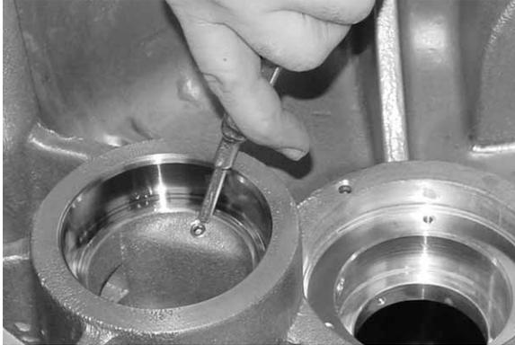
Install all plugs and install the lube pump in the bearing plate.
