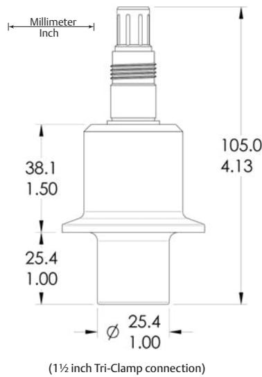
Figure 3. Rosemount 410VP-21 Conductivity Sensor dimensional drawing
