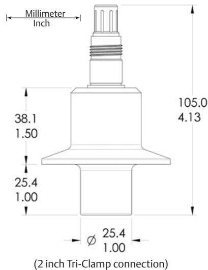
Figure 4. Rosemount 410VP-22 Conductivity Sensor dimensional drawing
