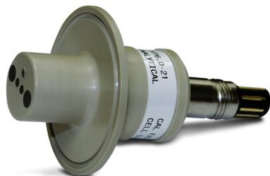
The Rosemount 410VP four-electrode conductivity sensor is intended for measuring conductivity in a variety of pharmaceutical and food and beverage applications. All wetted plastics and elastomers are compliant with 21CFR177, and all wetted surfaces except the electrodes have a 16 micro-inch (0.4 micrometer) Ra surface finish. A certificate of conformance is provided with each sensor. Interconnecting VP8 cable must be ordered separately and is required for all first time installations.
