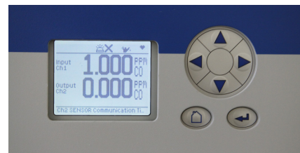
The enlarged graphic display of the X-STREAM Enhanced provides measurement and status information with plain text and symbols.
