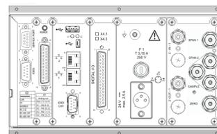
Rear panel layout with DC supply, USB, Ethernet, valve block and optional digital I/O board (rack version).
