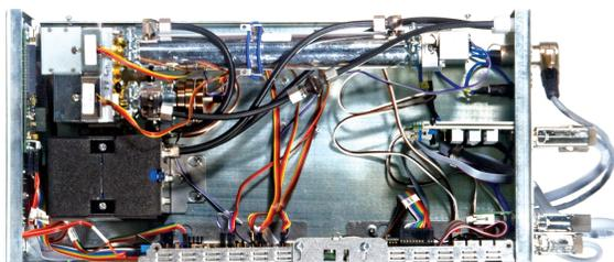
Interior view, showing one NDIR, one NDUV bench, one paramagnetic O<sub>2</sub> cell, analog and relay outputs, digital inputs, and serial interface.
