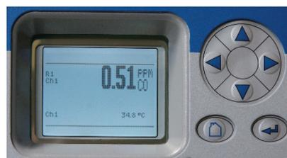
The enlarged graphic display of the X-STREAM Enhanced provides measurement and status information with plain text and symbols.
