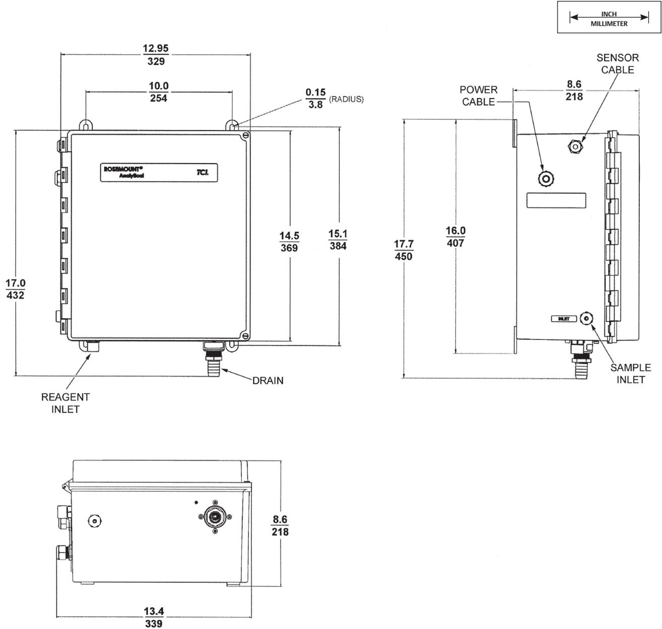
**Figure 2. Rosemount 1056-24 Panel Mount Installation**
