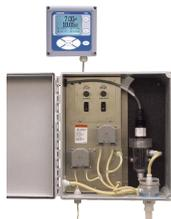
The Rosemount TCL total chlorine system consists of a sample conditioning system, a reagent carboy, a sensor, and a transmitter. Reagent kits for 0 to 5 ppm and 0 to 10 ppm chlorine ranges are available and must be ordered separately (see Accessories).
