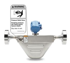
The sensor must be oriented so that personnel and equipment will not be exposed to any discharge along the pressure relief path. Stay clear of the rupture disk pressure relief area. High-pressure fluid escaping from the sensor can cause severe injury or death.
