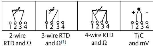
1. Emerson provides 4-wire sensors for all single element RTDs. You can use these RTDs in 3-wire configurations by leaving the unneeded leads disconnected and insulated with electrical tape.
