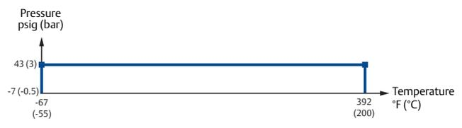
1. For antenna type code CAB, at 100 °F (38 °C), the rating decreases with increasing temperature per ASME B16.5 Table 2-2.2, Class 300.
