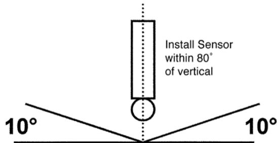
Figure 2. Dimensional Drawing for the Rosemount 3900/3900VP Sensor
