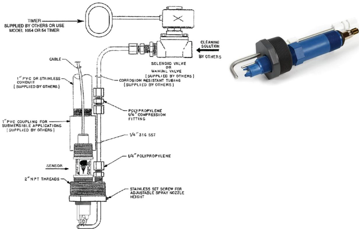
The jet spray cleaner eliminates routine, manual sensor maintenance by cleaning the sensor with water or compressed air. Flow through the cleaner can be controlled by a solenoid valve.
