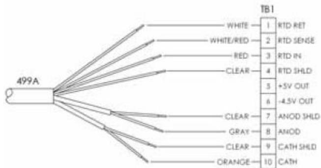
**Figure 4-5: Wiring Sensor with Standard Cable to Rosemount 56 Transmitter**
