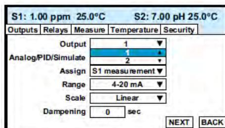
7. To view the list, press and hold **Up** or **Down**. To select and store the highlighted selection, press **ENTER/MENU**. To move from one control box to another, press **Up** or **Down**.
