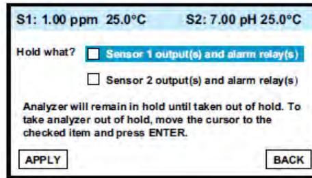
3. To hold outputs and relays associated with sensor 1, press **ENTER/MENU**. A check appears in the checkbox. To put sensor 2 on hold also, move the cursor to the sensor 2 line and press **ENTER/MENU** to select the sensor 2 checkbox.
