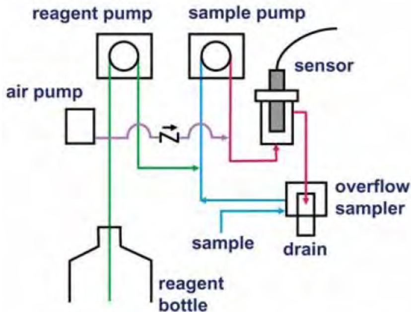
The treated sample next enters the flow cell. Bubbles injected into the flow cell produce turbulence, which improves the stability of the reading. A membrane-covered amperometric sensor in the flow cell measures the concentration of iodine. The transmitter receives the raw signal from the sensor and displays the concentration of total chlorine. Display units are ppm (mg/L) chlorine as  $\text{Cl}_2$ . The treated sample leaves the flow cell and drains to waste along with the excess sample.
