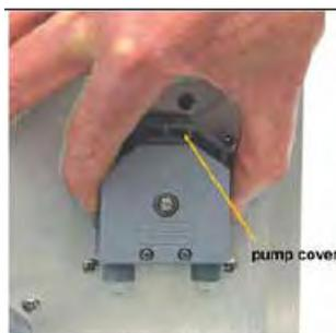
4. Using your thumb as shown in [Figure 12-7](#), push the tubing fitting straight outward until the fitting slides out of the socket.
