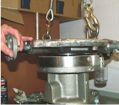
Seal housing with bearing box shown.
