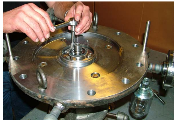
Tightening the bolts on the lower process seal.
