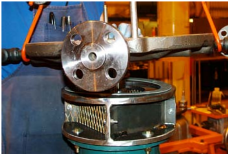
Seal housing with extended motor shaft adapter shown.
