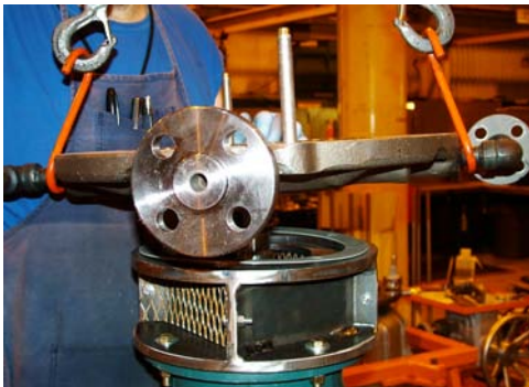
Seal housing being installed onto extended motor shaft adapter.
