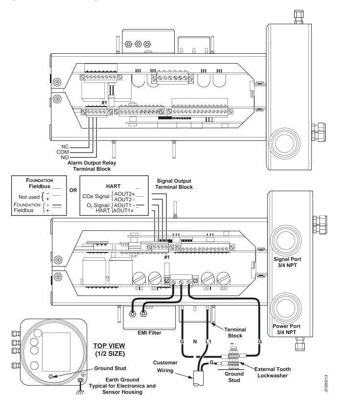
Figure 9-6. Remote Electronics Housing Cable Connections
