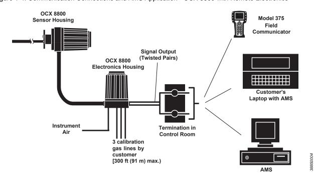
Figure 1-5. Typical System Installation - Integral Electronics
