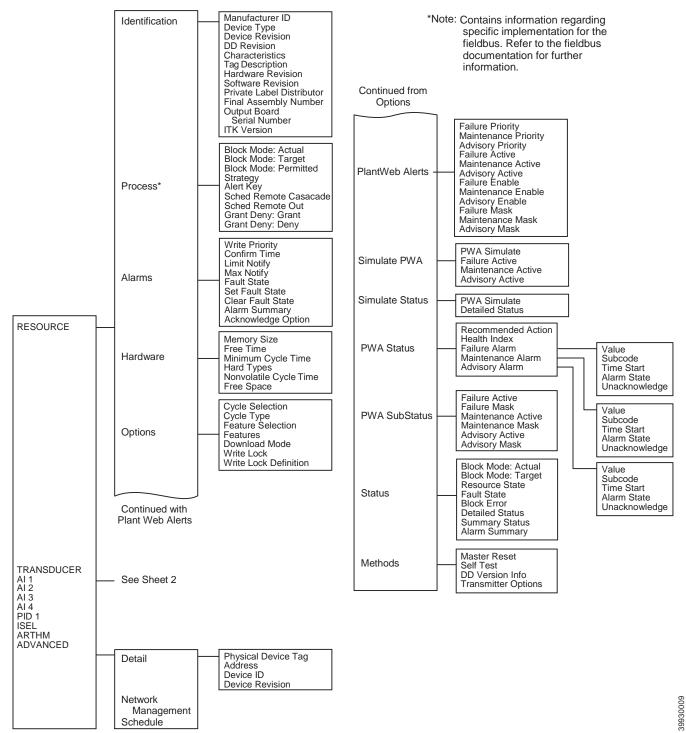
Figure 6-8. Fieldbus Menu Tree (Sheet 2 of 3)
