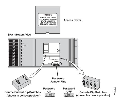
Figure B-4. SPA Setup for Calibration
