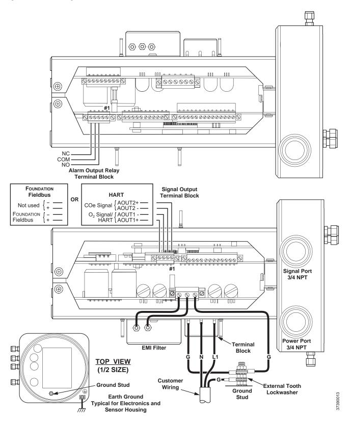
Figure 2-7. Electrical Connections Between Remote Electronics and Sensor Housing SHIELD YEL 2HTR CO RED 1HTR CO BLK 2HTR O<sub>2</sub> ORG 1HTR O<sub>2</sub> To WHT 2HTR SB ground BLU 1HTR SB screw Heater Power Connector (J3) 000 000 000000000 0000000  $^{\scriptsize{\scriptsize{\scriptsize{\scriptsize{(}}}}}$ (H) **RED** T/C CO+ T/C CO-0000 **BLK** WHT T/C SB+ Heater Power Cable BLK T/C SB-GRN YEL T/C O2+ EXC+ BRN | T/C O2-CO ACT+ BLK CO ACT-O2 CELL+ **COe Sensor** BLK and
