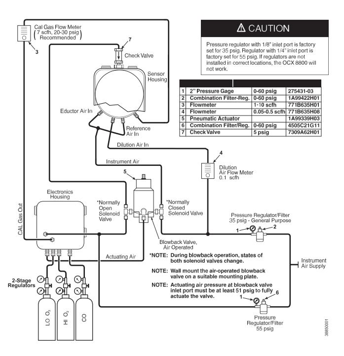
Figure 2-13. Pneumatic Installation, OCX with Reference Air Set, Solenoids, Blowback and Autocalibration, with COe Zero Function
