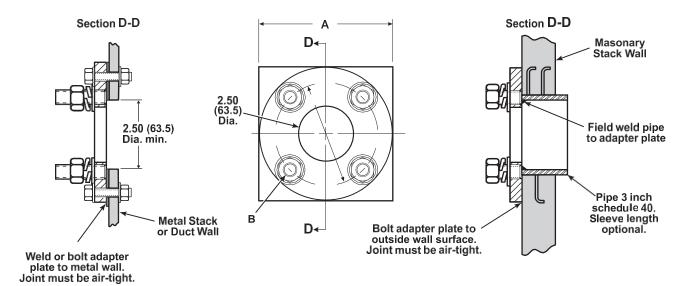
METAL WALL STACK OR DUCT CONSTRUCTION MASONRY WALL STACK CONSTRUCTION
