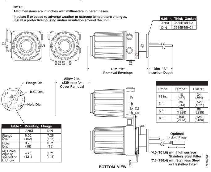
Figure 2-2. Installation, OCX 8800 with Remote Electronics
