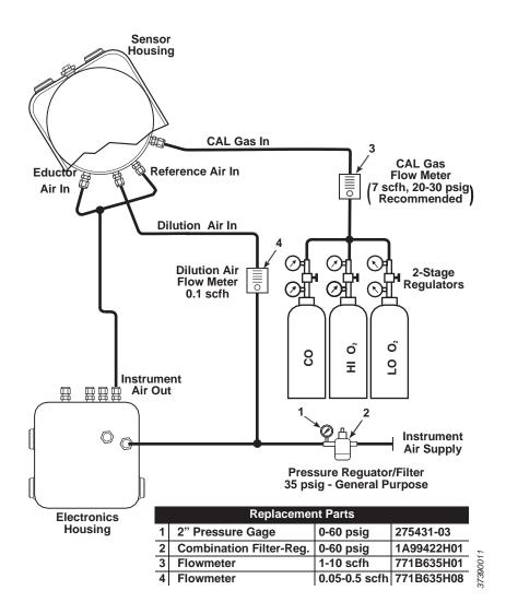
Figure 2-10. Pneumatic Installation, OCX with Reference Air Set, Solenoids and Autocalibration, without COe Zero Function
