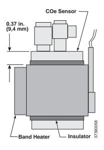
Figure 9-20. COe Sensor Holder Alignment
