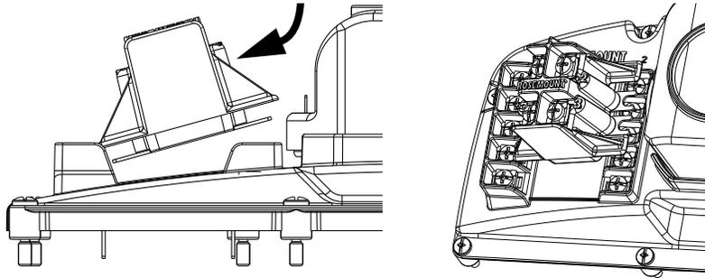
3. Lower right side of adapter into terminals 2 and 3 on the right side and center the adapter.
