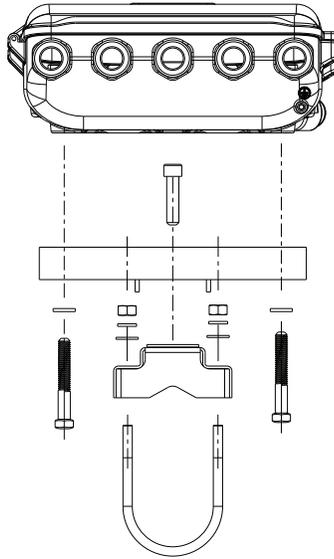
3. Run wiring (and conduit, if necessary) from the sensor to the 848T. For an easier installation, use the outside conduit entries, as shown below. Any unused conduit entries should be sealed with an approved sealant using the included threaded conduit plug.
