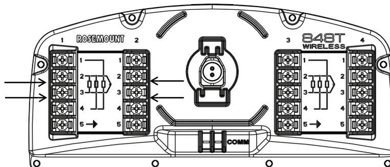
2. Angle adapter and slide spade lugs into terminals 2 and 3 on the left side, as shown in the figure below. Ensure that the positive and negative polarity indicators match on the adapter and the terminal block.
