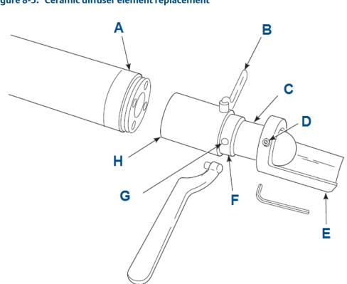
Figure 8-5: Ceramic diffuser element replacement
