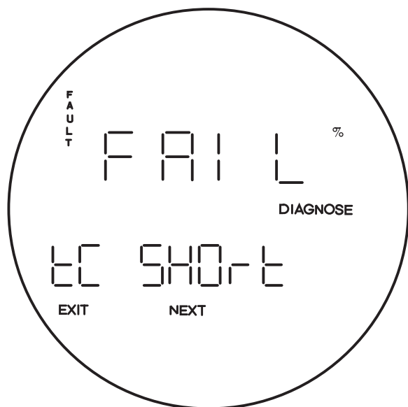
Figure 5-7. Fault 3, Shorted Thermocouple
