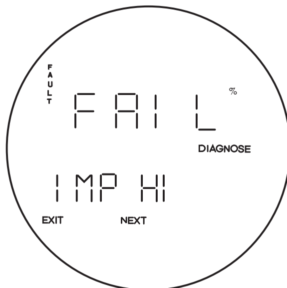
Figure 5-10. Fault 6, Cell Impedance Too High
