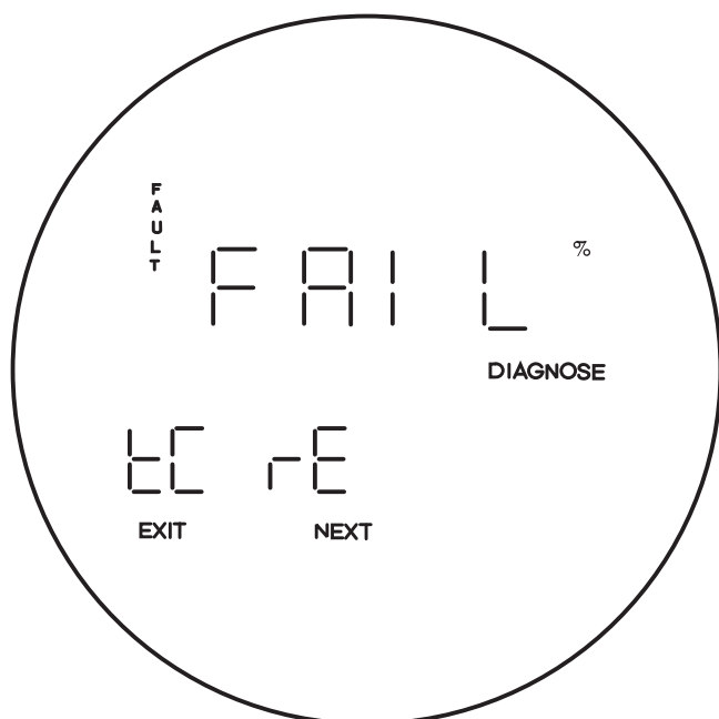
Figure 5-6. Fault 2, Reversed Thermocouple
