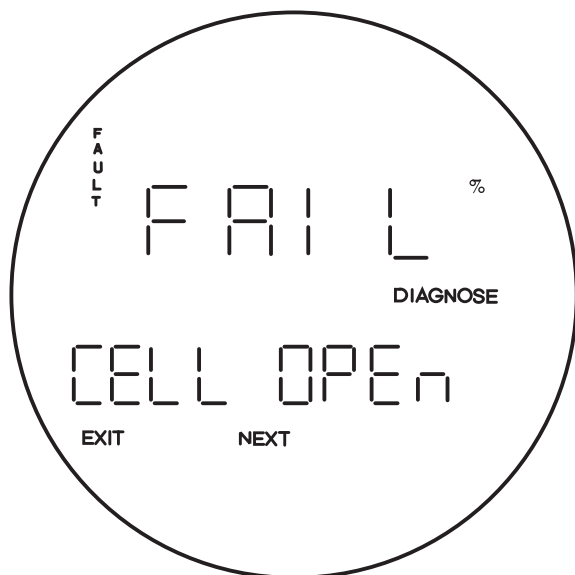
Figure 5-9. Fault 5, O 2 Cell Open
