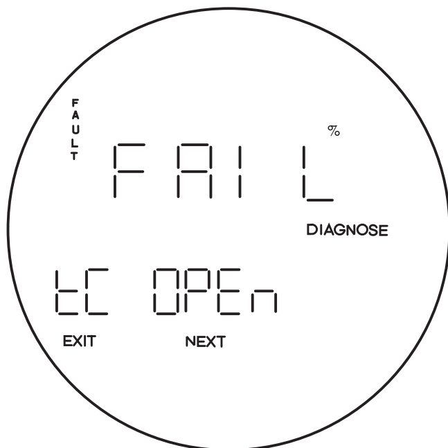
Figure 5-5. Fault 1, Open Thermocouple
