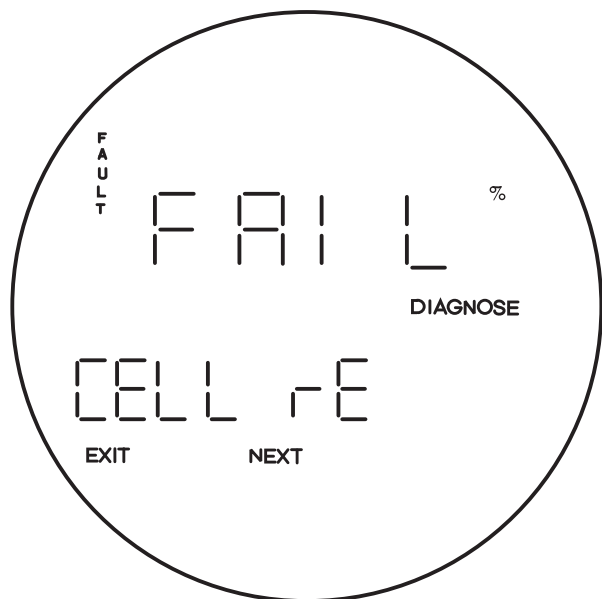
Figure 5-11. Fault 7, Reversed O 2 Cell
