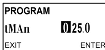
4. Use the arrow keys to change to the desired temperature. To enter negative numbers, press the left or the right arrow key until no digit is flashing. then press the up or down arrow keys to display the negative sign.
