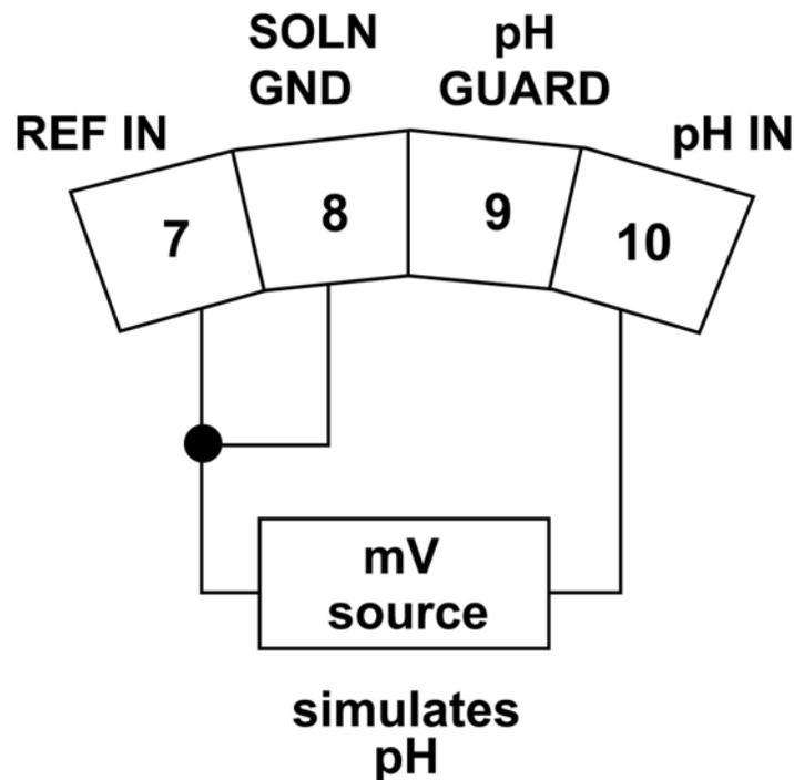
6. Calibrate the transmitter. Use 0.0 mV for Buffer 1 (pH 7.00) and -177.4 mV for Buffer 2 (pH 10.00).
