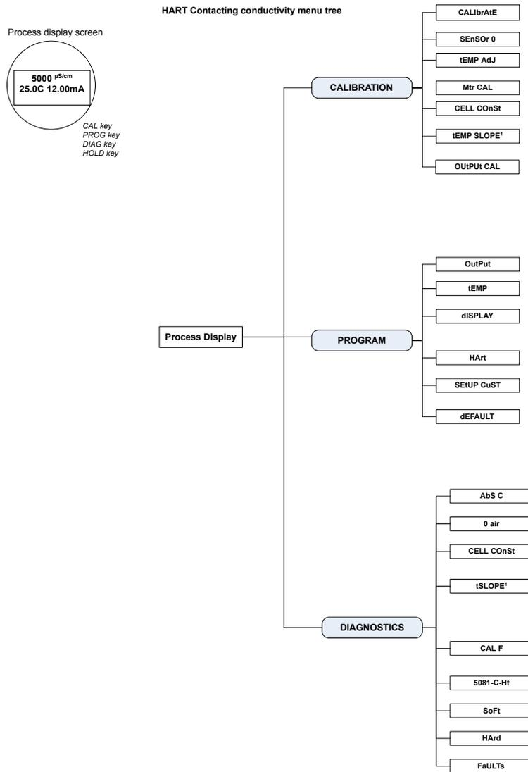
Figure 5-7: HART toroidal conductivity menu tree
