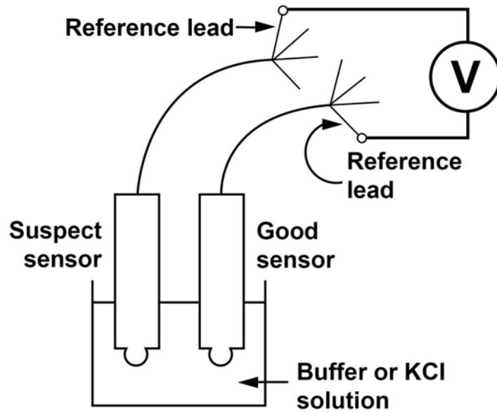
Refer to the sensor wiring diagram to identify the reference leads. A laboratory silver/silver chloride electrode can be used in place of the second sensor.
