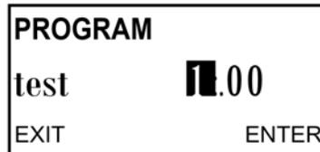
11. Use the arrow keys to enter the desired test current. Press *ENTER* to start the test. Press *EXIT* to end the test.
