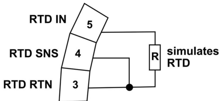
The figure shows wiring connections for sensors containing a Pt 100 RTD. For sensors using a 22k NTC thermistor (Hx438 and Gx448 sensors), wire the decade box to terminals 1 and 2 on TB6.
