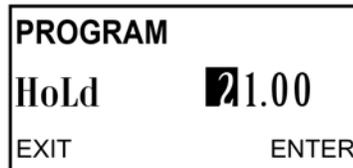
5. Use the arrow keys to change the setting to the output desired when the transmitter is in hold mode.
