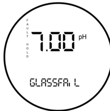
*When a disabling condition, a fault, occurs, the display appears as pictured above. To further alert you that measurements are in error, the display flashes. Diagnostic messages appear in the temperature/output area on the screen.*
