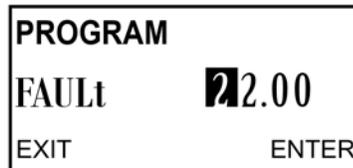
7. Use the arrow keys to change the setting to the output desired when the transmitter is in fault mode.
