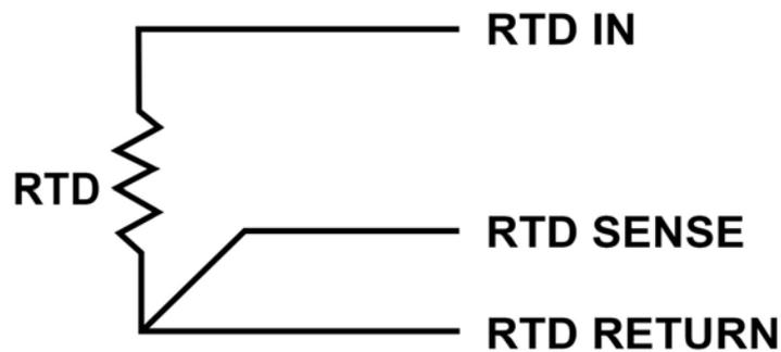
Although only two wires are required to connect the RTD to the analyzer, using a third wire allows the analyzer to correct for the resistance of the lead wires and for changes in the lead wire resistance with temperature.
