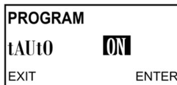
3. Use the up or down arrow keys to enable (**ON**) or disable (**OFF**) the automatic temperature correction feature. Press *ENTER* to save.
