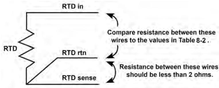
Consult the table for resistance-temperature data. Lead resistance is about 0.05 ohm/ft at 25 °C. Therefore, 15 feet of cable increases the resistance by about 1.5 ohm. The resistance between the RTD return and RTD sense leads should be less than 2 ohms.
