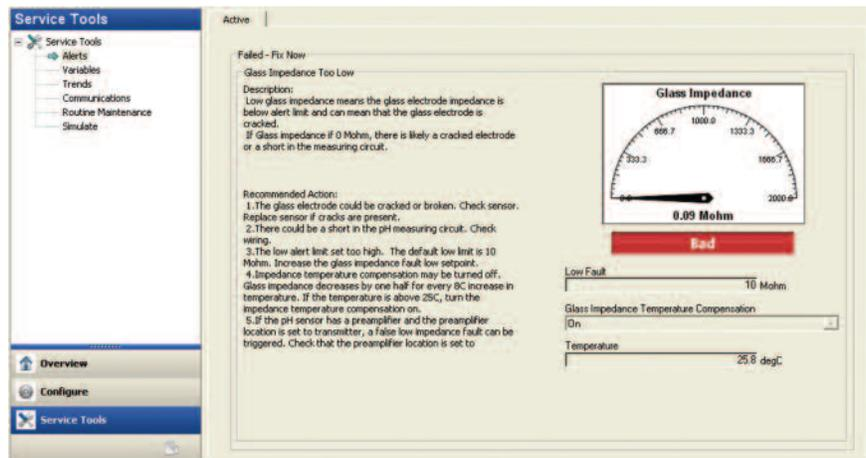
In addition to providing notification of sensor and transmitter conditions, diagnostics alerts also affect the status of the measurements affected by the conditions to provide a means to inform the control system of the validity the measurements it is acting on. These effects on status can be summarized below:
