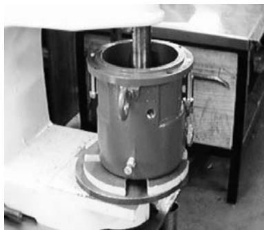
Figure 11-16: Install Labyrinth Seal into Cavity
