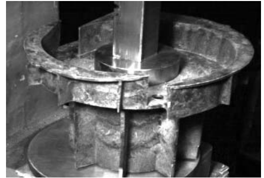
Figure 9-2 Shaft support into volute
