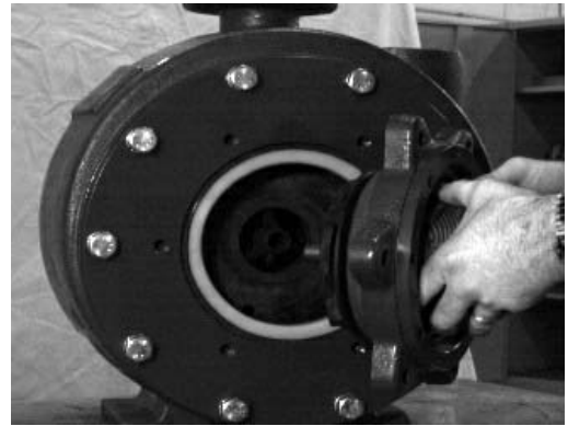
Figure 9-10 Assembling impeller/rear casing
