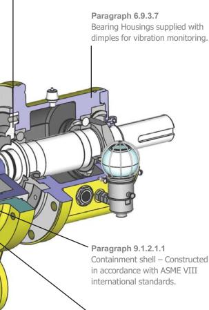
**Paragraph 6.10.8** Thrust bearings – Designed for capacity in both directions.
