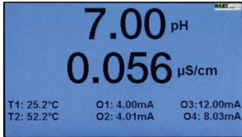
**Quick Start Programming:** Simple Quick Start screens appear the first time the unit is powered. The instrument auto-recognizes each type of measurement board and prompts the user to configure each sensor loop in a few quick steps for immediate live readings.
