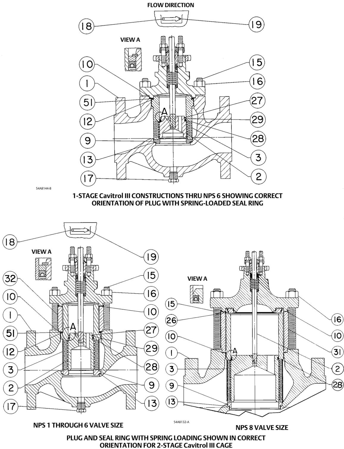
Figure 21. Gasket Set Detail shown with Optional Drain Plug
