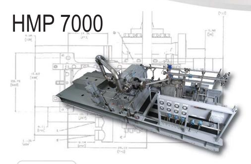
The **HMP-7000** is a three-stage centrifugal process pump.
