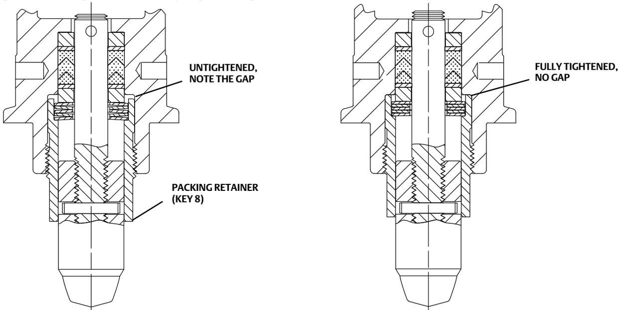
BELLEVILLE SPRINGS FULLY ENCLOSED BY THE PACKING RETAINER
