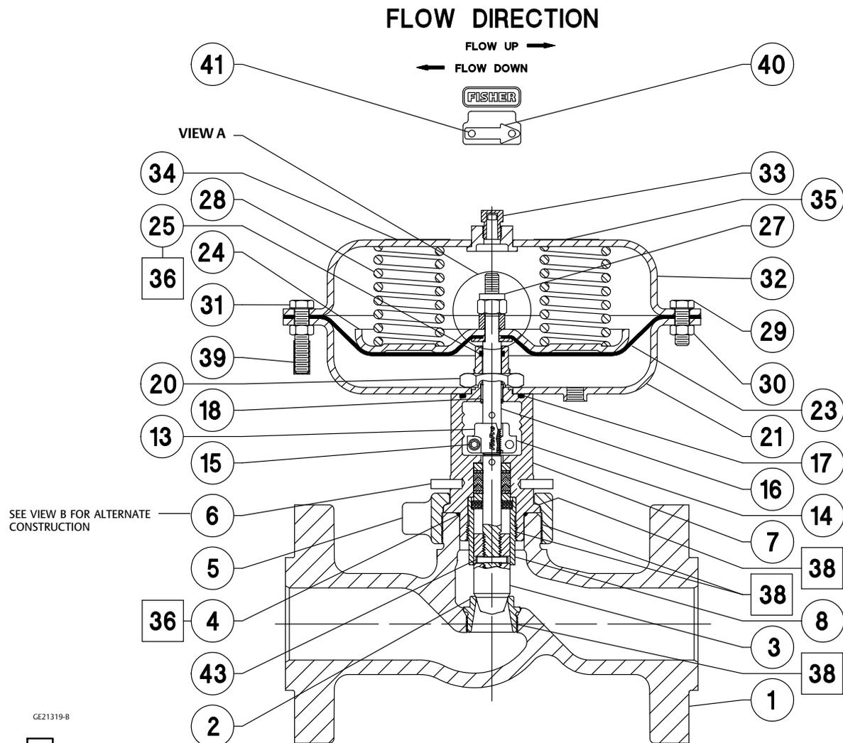
Figure 8. Fisher D3 FloPro Valve Assembly (Spring-to-Open)
