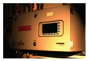
Rosemount Analytical's MLT2 offers multi-component, multi-method analysis utilizing infrared, visible, ultraviolet, thermal conductivity, paramagnetic, and electrochemical sensor technologies, as well as trace oxygen and moisture.
