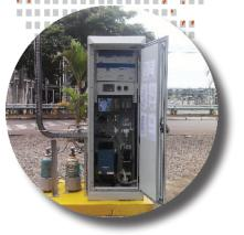
The continuous emissions monitoring package with X-STREAM general purpose gas analyzers performs self-diagnostics and is fully pre-engineered for maximum uptime. The system can measure up to four of the following gas constituents: O<sub>2</sub>, CO, CO<sub>2</sub>, SO<sub>2</sub>, NO, NO<sub>2</sub>, and NOx. Opacity can be measured with the addition of an opacity monitor.
