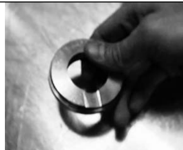
Fig. 12-13: Labyrinth Seal w/ Port at 6 o'clock
