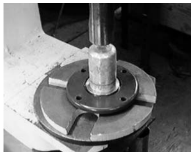
Fig. 12-14: Install Labyrinth Seal in Bearing Cap
