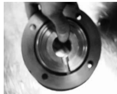
Fig. 12-15: Labyrinth Seal in Bearing Cap
