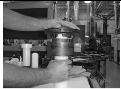
Figure 7-14: Separation of the impeller and inner drive
