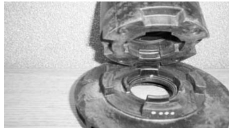
Figure 9-8 Placing back plate on casing
