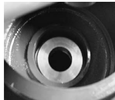
Fig. 11-17: Labyrinth Seal in Cavity
