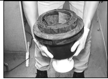
Fig. 7-17: Magnet removal tool placed in bushing bore
