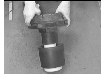
Fig. 7-18: Inner magnet and impeller separated
