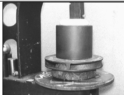
Fig. 8-4: Inner magnet assembly and impeller form single unit
