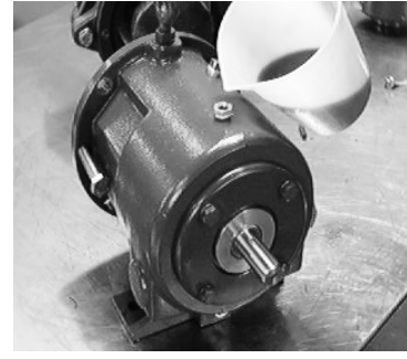
Fig. 12-22: Fill Bearing Frame with Oil
