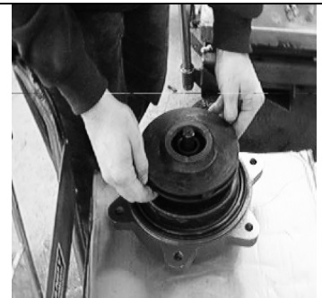
Fig. 7-10: Remove Impeller from Containment Shell
