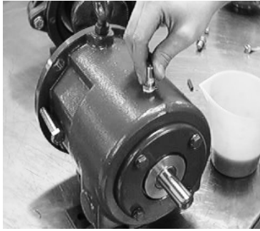
Fig. 12-21: Remove Breathing Tube
