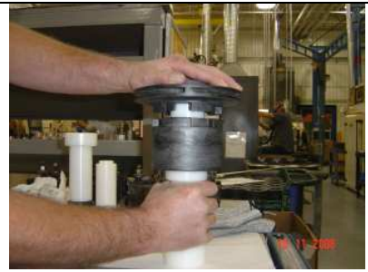
Figure 7-14: Separation of the impeller and inner drive
