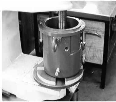
Fig. 12-16: Install Labyrinth Seal into Cavity
