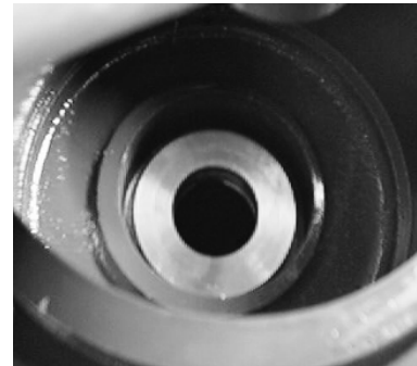
Fig. 12-17: Labyrinth Seal in Cavity
