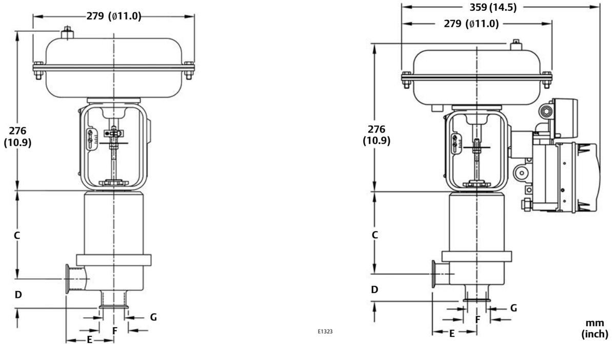
NOTE: ACTUATOR REMOVAL REQUIRES 115mm (4.5 INCHES) VERTICAL CLEARANCE. FOR PROPER ADJUSTMENTS TO DUAL TRAVEL STOPS, REFER TO ACTUATOR INSTRUCTIONS
