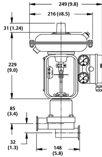
84000 INLINE VALVE BODY WITH BAUMANN 32 ACTUATOR ATC/FO ACTION, DUAL STOP AND 3660/3661 POSITIONER
