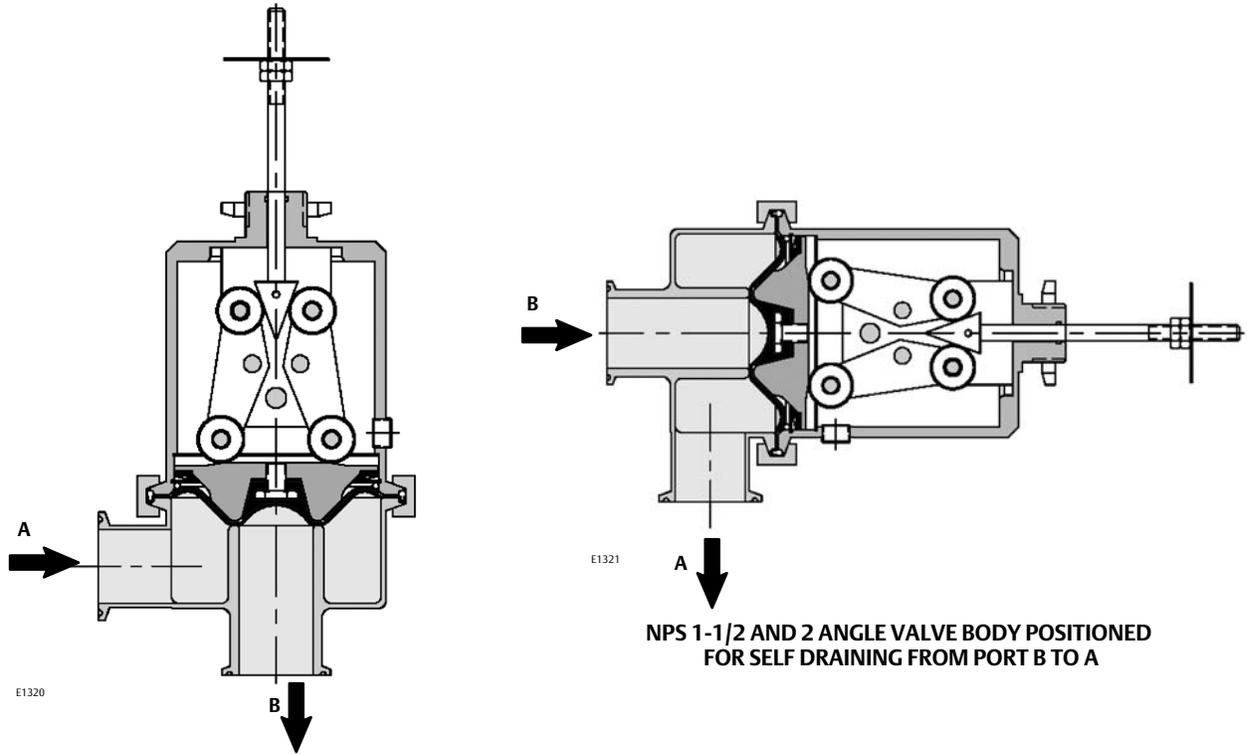
NPS 1-1/2 AND 2 ANGLE VALVE BODY POSITIONED FOR SELF DRAINING FROM PORT B TO A
