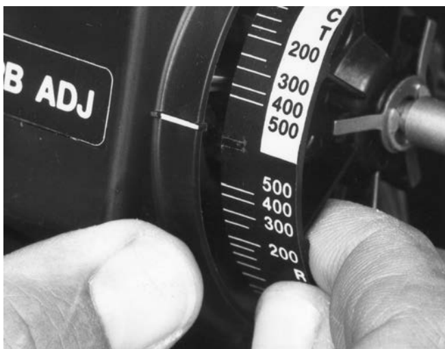
Figure 24. Changing Controller Action (Fisher 4196S Controllers)
