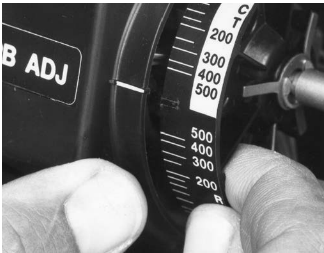
Figure 15. Fisher 4196B and C Controller Changing Controller Action
