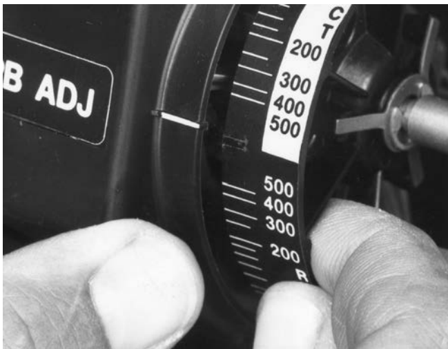
Figure 10. Fisher 4196A Controller Changing Controller Action
