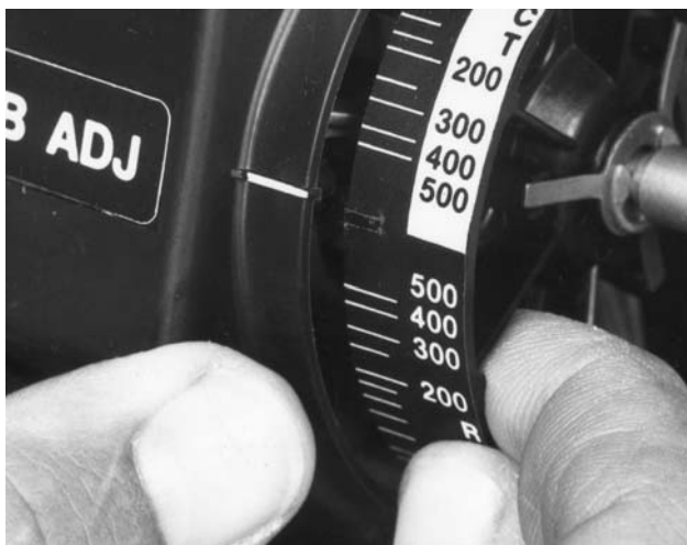
Figure 4-3. Changing Controller Action (Fisher 4194B and C Controllers)
