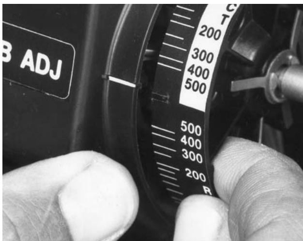
Figure 3-2. Changing Controller Action (Fisher 4194A Controllers)
