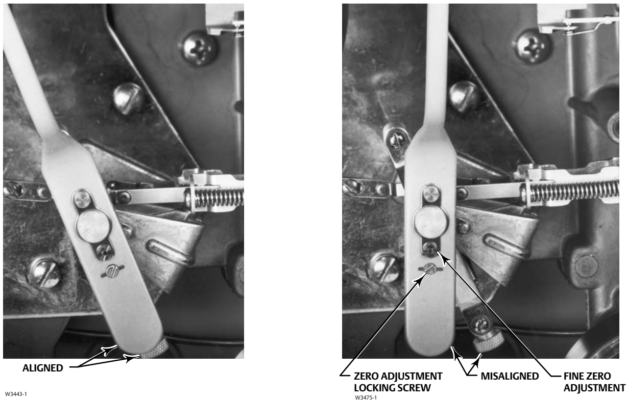
Figure 5-14. Process Pointer Alignment
