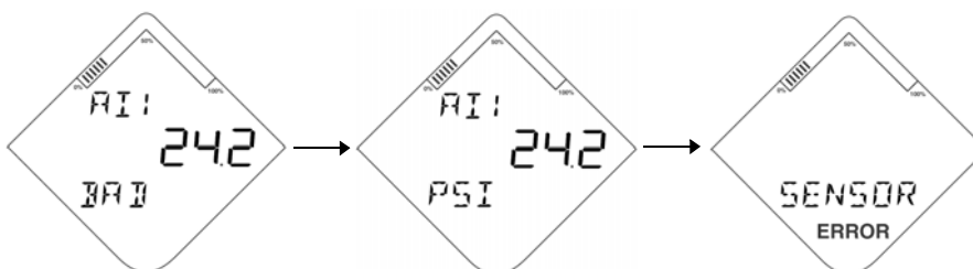
Figure 3-4. LCD Display Messaging
