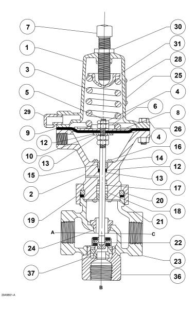
Figure 3. Type 122A Three-Way Switching Valve Assembly
