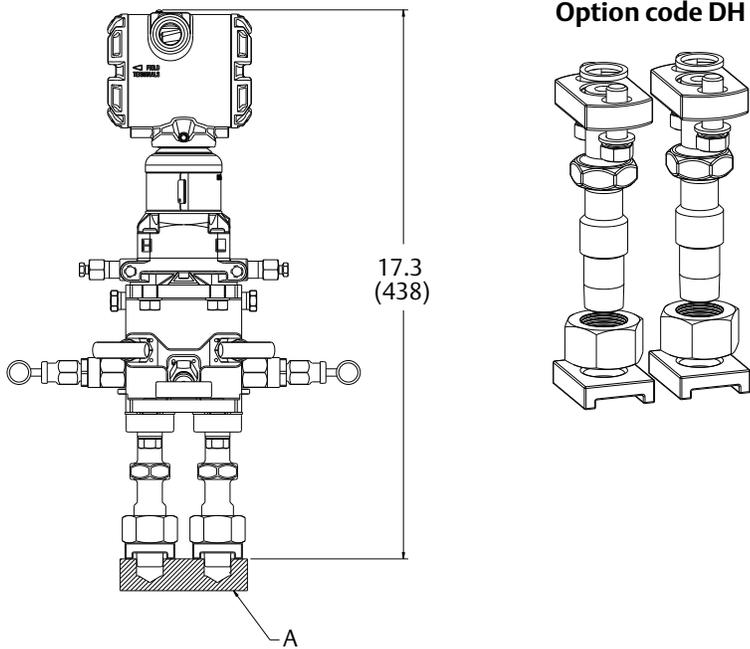
A. Cross section image is shown for dimensioning purposes only; it is not part of the transmitter assembly
