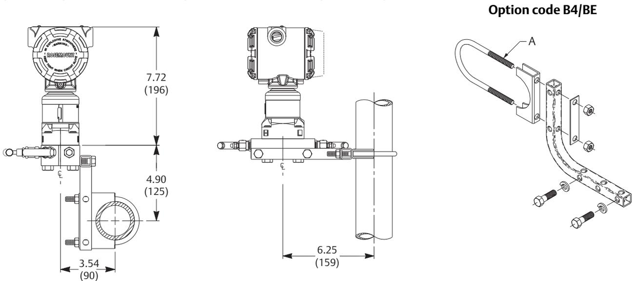
A. 2-in. U-bolt for pipe mounting
